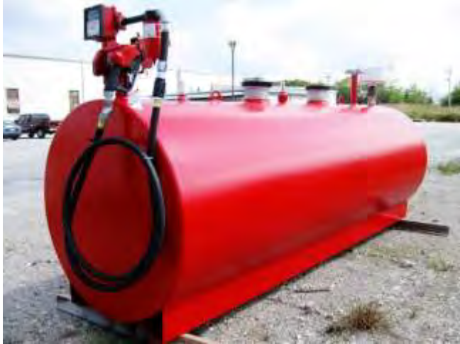
Photo 2: Typical 1000-gallon double walled fuel tank. These tanks will be on the barges and used for filling the equipment running at a given operation.
