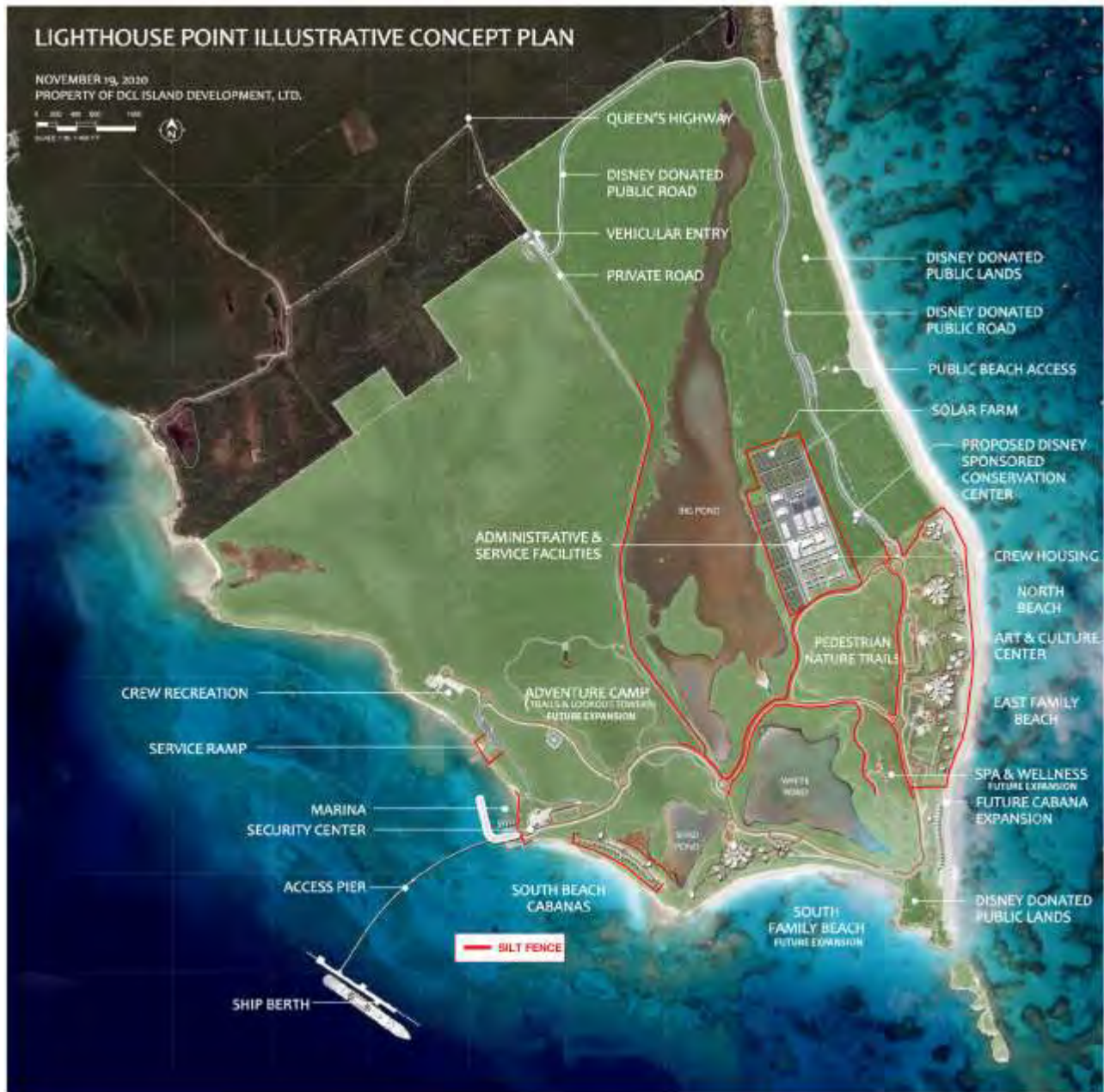
Figure 4: Planned Silt Fence Installation Locations at Lighthouse Point
